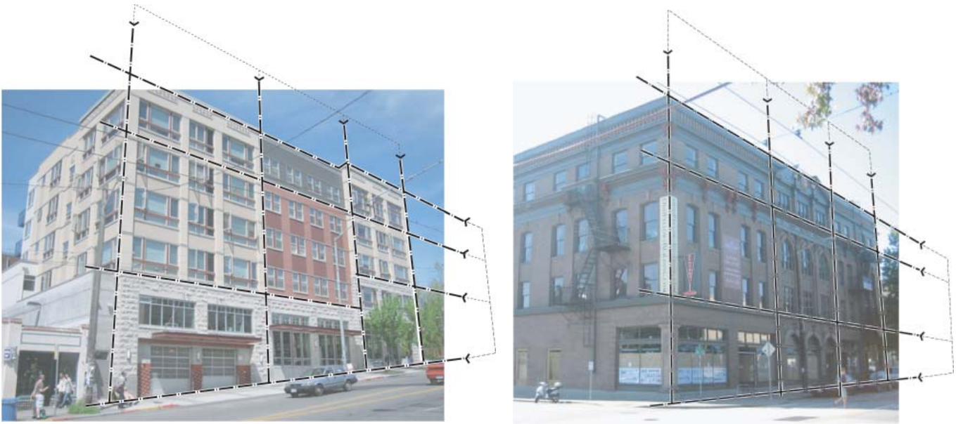
Figure 9: The rhythm established by the neighborhood's original platting and early development provides the basis for determining an appropriate scale relationship between new and old. These illustrations show how the vertical and horizontal treatment of the facades in both an older and more recent building express the prevailing width and height patterns in larger structures.
